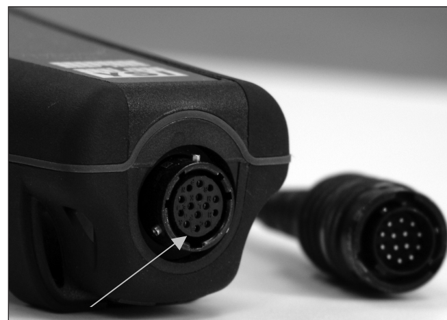
Figure 4, Note the keyed connector.
